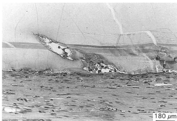
Figure 5 Macrophages and giant cells were clearly involved in the fragmentation process of the polymer surface in the cracks and voids.
